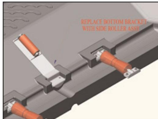
5. Reattach the original roller without the bottom bracket.
