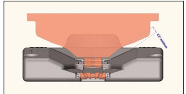
Before Disassembling the rollers check that there is enough room to fit the stabilizer rollers by inserting them in the gap as shown below. There will be enough room if the conditions above are met.
